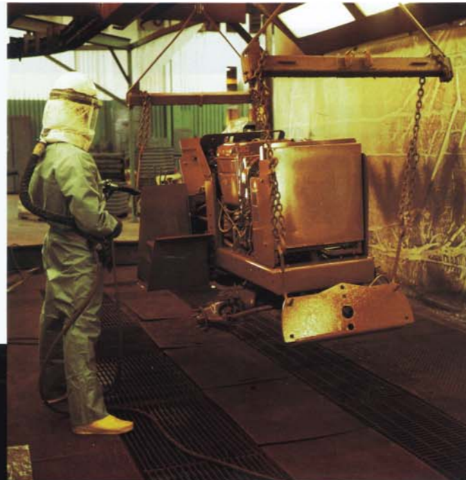
Ditch Witch products' bright orange paint is applied just before the final assembly process. Some painting may be moved closer to the assembly line as part of the company's focused factory approach.
