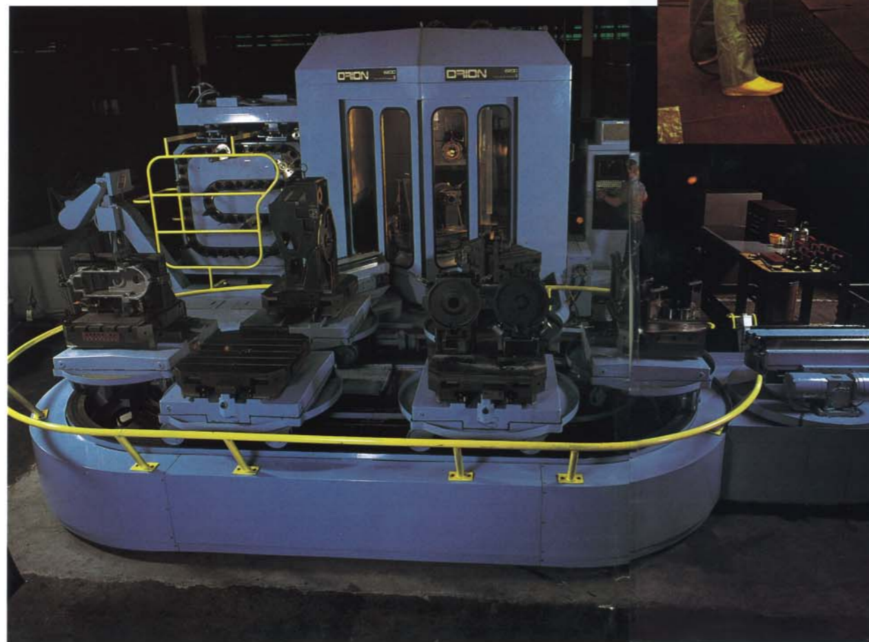
This computerized multiple machining center has 150 tools and eight pallets for making gearboxes. This cell includes two assembly stations, a washer and deburrer, so when a gearbox leaves on color-coded racks, it's ready to bolt onto a machine.
